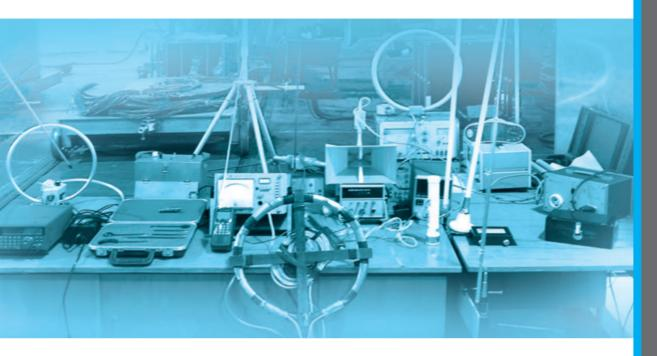
The Krylov State Research Centre has developed a mobile instrumentation system for measuring the electromagnetic compatibility (EMC) parameters of full-scale electronic & electric systems on industrial sites and transport vehicles, as well as test benches of equipment manufacturers. EMC tests can be performed in parallel with the trials of the main equipment functions.
