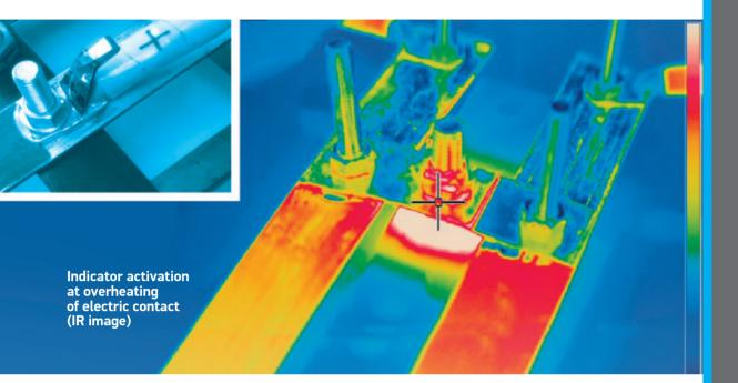
The overheating indicators are helpful tools in reducing the electric equipment fire hazards by detection of contact overheating during scheduled maintenance of shipboard electric equipment.
