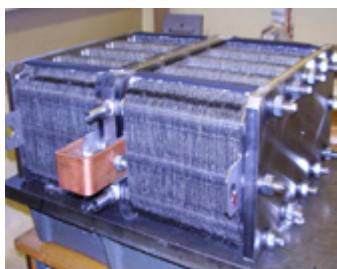
PEM fuel cell battery working on synthesis gas and air. The electrical power is 6,5 kW
