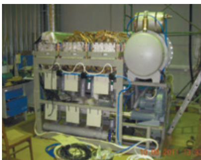
Combined power plant with electrical power of 60 kW. The high efficiency is attained as a result of including of gas-turbine generator in the power plant with electrochemical generator based on PEM fuel cells. Diesel oil is initial fuel
