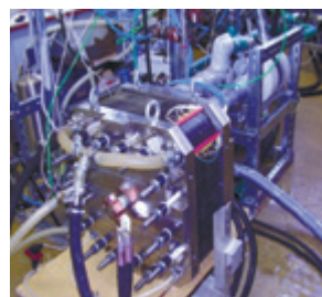
Test of PEM fuel cell battery prototype working on purified synthesis gas and air, area of fuel cell active surface is 1225 sq.cm
