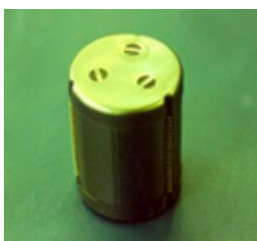
Intermetallic accumulator of hydrogen based on the alloy \text{LaNi}_5 is the safest and most compact ( 800 \text{ nl H}_2/\text{dm}^3 ) system of hydrogen storage
