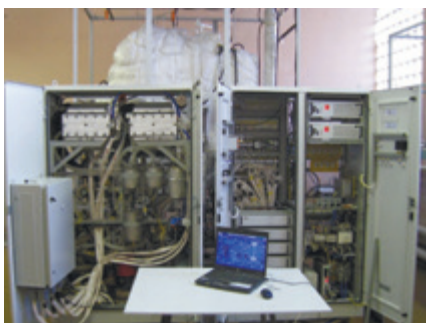
Cogeneration power plant based on PEM fuel cells working on natural gas. The electrical power is 10 kW
