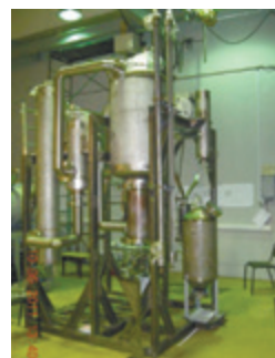
Combined power plant with electrical power of 60 kW. The high efficiency is attained as a result of including of gas-turbine generator in the power plant with electrochemical generator based on PEM fuel cells. Diesel oil is initial fuel
